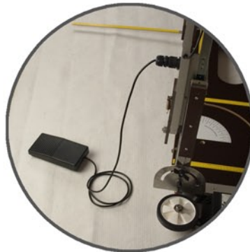
The foot operated switch is attached to the cutting bow.
